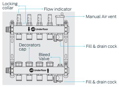
When initially filling the UFH heating system it is important to remove the air in the pipework.
