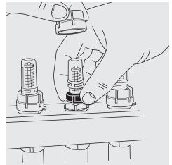
Each flow meter comes with an indicator sleeve, these can be positioned to correspond with the flow rate which has been set for each one.
