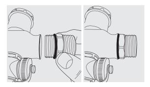
3. Connect the two way union to the male thread of the adapter that you have just screwed into place. Take care to insert the washer in between the flat faces. It is important that the ridgid end be connected to the threaded part and the free spinning nut be left to connect to the new manifold extension.
