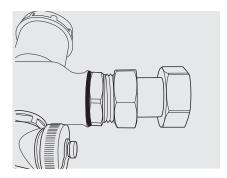
4. Connect the free spinning nut to the inlet thread of the new manifold you are adding on making sure to include the washer for the flat faced connection.
